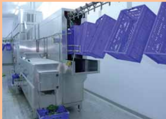
Overhead crate washer
