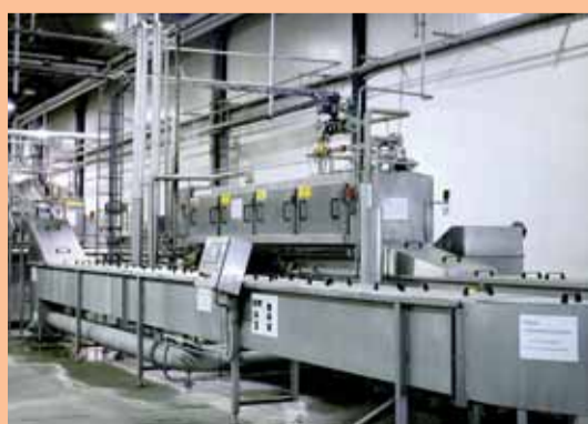
Crate washer with soaking section for extreme soiling
